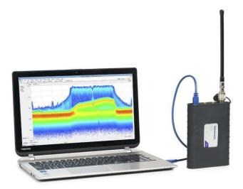
The RSA306 uses your PC and Tektronix SignalVu-PC<sup>™</sup> RF Signal Analysis Software to provide real time spectrum analysis, streaming capture and deep signal analysis capabilities for signals from 9 kHz to 6.2 GHz, all in a low-cost, highly portable package that is ideal for field, factory, or academic use.
