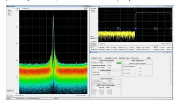
Sophisticated WLAN measurements are easy. On the following 802.11g signal display below, the spectrogram shows the initial pilot sequence followed by the main signal burst. The modulation is automatically detected as 64 QAM for the packet and displayed as a constellation. The data summary indicates an EVM of -33.24 dB RMS, and burst power is measured at 10.35 dBm. SignalVu-PC applications are available for 802.11a/b/j/g/p, 802.11n and 802.11ac to 40 MHz bandwidth.
